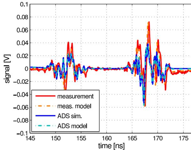
Figure 3.13: Time domain output signals of the nonideal multiplier system model in comparison to the measurement, the output signal of the ADS circuit model, and the system model fitted onto the ADS circuit model.
