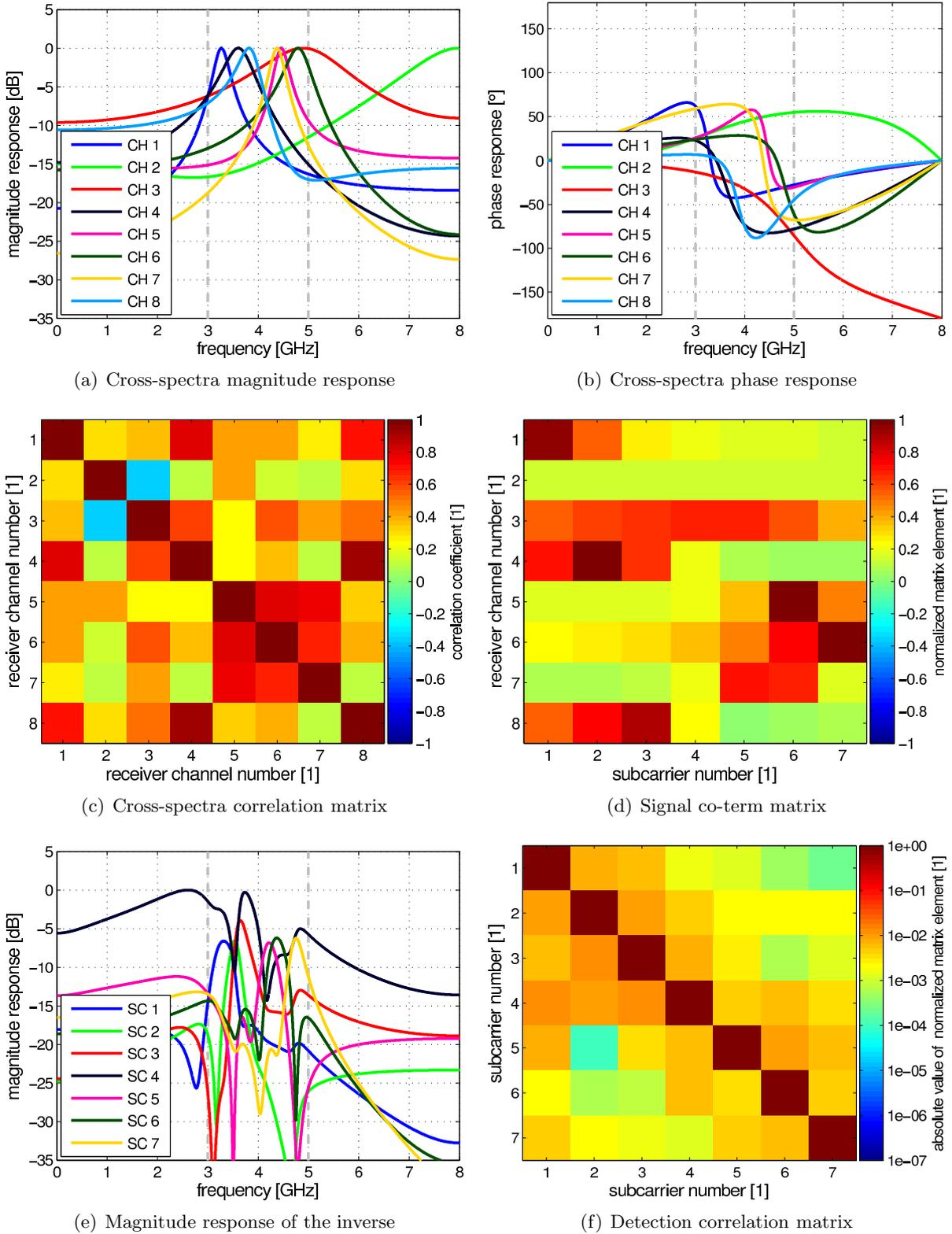
Figure 3.2: Frequency response, Correlation matrix, and signal co-term matrix  $\mathbf{P}$  of a projection filter cross-spectra of 2<sup>nd</sup> order. The shown cross-spectra do have a condition number of  $\text{cond}\{\mathbf{P}\} = 19.48$ .
