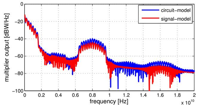
Fig. 5. Frequency domain output signals of the nonideal multiplier model in comparison to the output signal of the circuit model of five NOFDM pulses. The input signals had a power of  $-20$  dBm.
