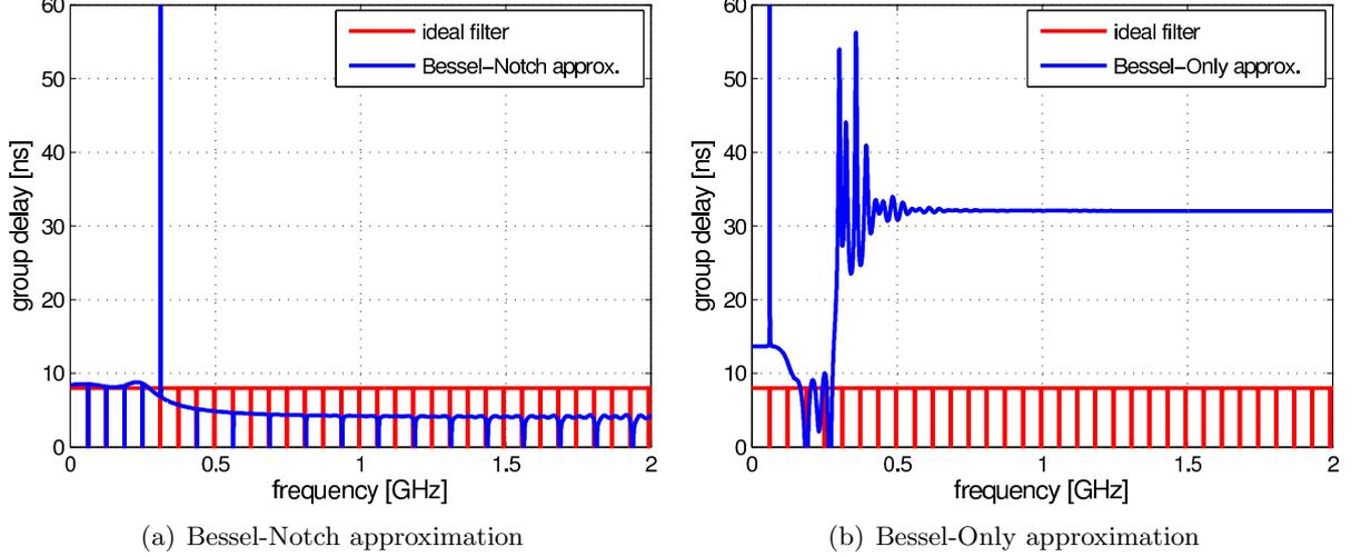
Figure 3.21: Group delays of the Bessel-Notch approximation and Bessel-Only approximation sliding window integrator with 8<sup>th</sup> filter order.
