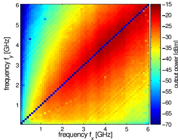
Figure 3.10: Magnitude response of two dimensional frequency sweep measurements. Each grid point represents the output power of the output single-tone at a frequency of  $|f_x - f_y|$ , where  $f_x$  and  $f_y$  are frequencies of the input single-tones.
