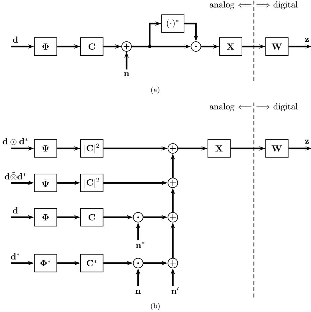
Figure 2.4: Two equivalent matrix signal flow diagrams of the generalized noncoherent multi-channel receiver.
