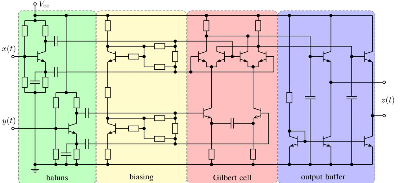
Fig. 2. Circuit model of the UWB mixer designed by Ulm University consisting of two active single-ended-to-differential converter input stages (baluns), biasing, a four-quadrant Gilbert cell multiplier, and an output buffer.
