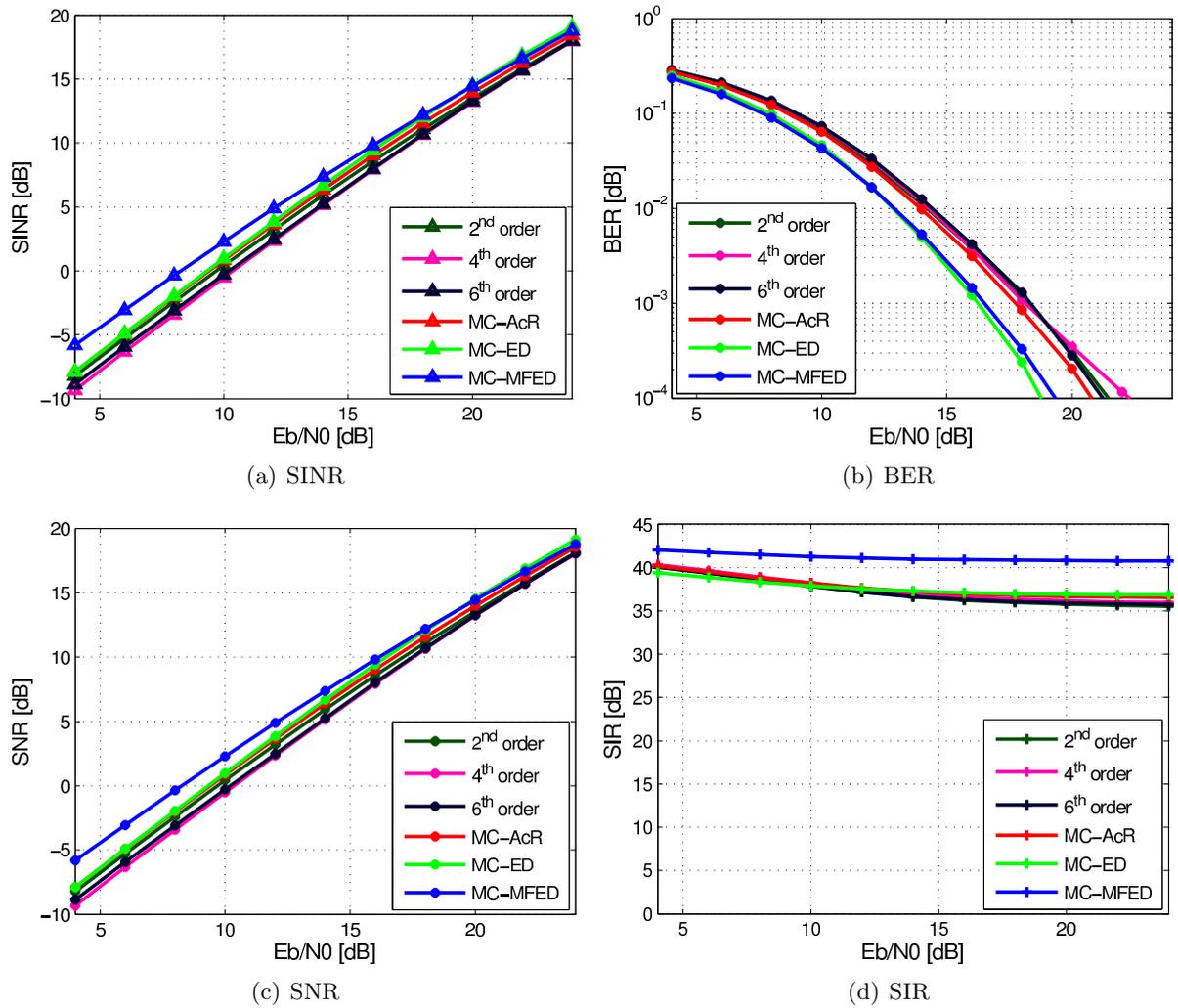
Figure 3.5: SINR, SNR, SIR, and BER of the generalized noncoherent multi-channel receivers with various orders of projection filter cross-spectra.
