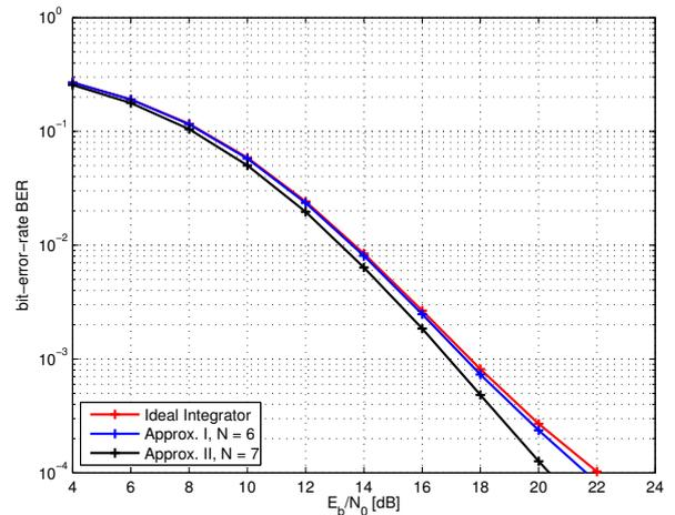
Fig. 5. BER for the given approximation setups in comparison to an ideal integrator.
