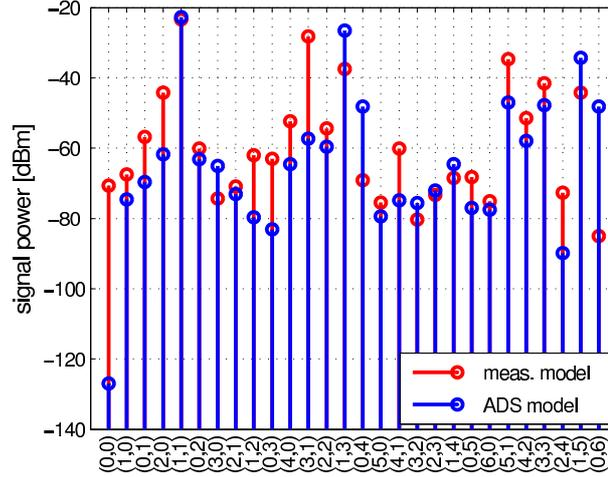
Figure 3.15: Power of the nonlinear signal with the respective coefficients  $\{c_{u-v,v}\}$  of the system model fitted to the measurement and the system model fitted to the ADS simulation. The pair  $(a,b)$  represents its respective nonlinear coefficient  $c_{a,b}$ .
