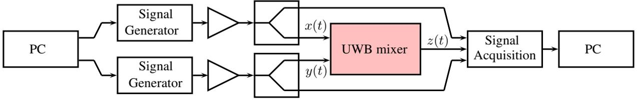
Fig. 4. Measurement setup for mixer identification.
