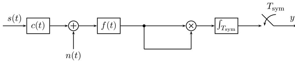
Figure 1.3: Signal flow diagram of an energy detector.
