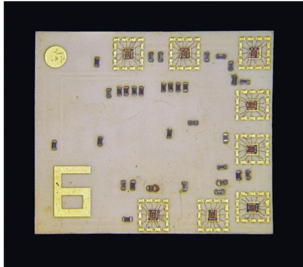
Figure 5.3: Photograph of the realized MC-AcR LTCC module with eight mounted UUm UWB mixers.
