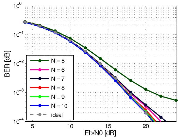
(b) BER of MC-AcR with Bessel-Notch filter approximation.
