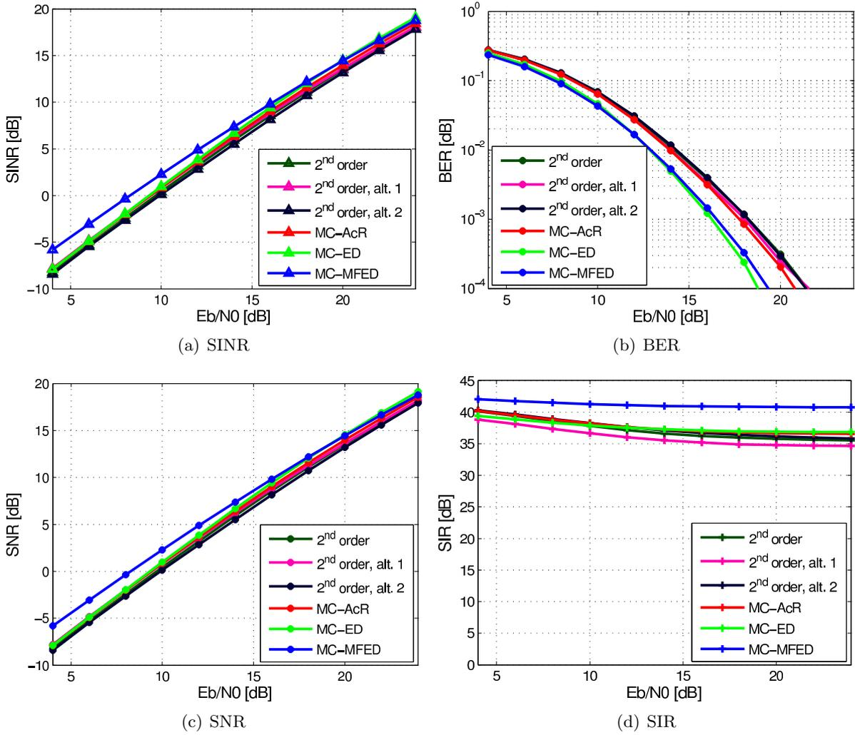
Figure D.4: SINR, SNR, SIR, and BER of the generalized noncoherent multi-channel receivers with various 2<sup>nd</sup> order projection filter cross-spectra.
