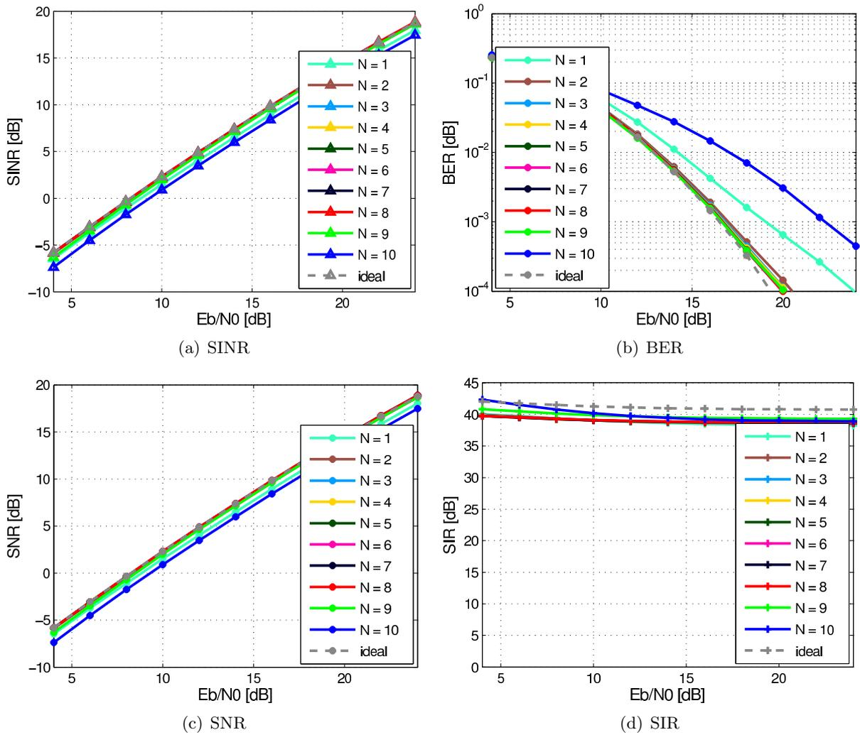
Figure D.13: SINR, SNR, SIR, and BER of the MC-ED with various filter orders  $N$  of Bessel-Only filter approximations.
