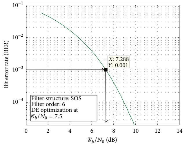
FIGURE 6: Transceiver BER for the optimum solution found by the DE algorithm. The operating point for fixed- and floating-point analysis is chosen to be at a BER of  $10^{-3}$  resulting in an  $\mathcal{E}_b/N_0$  ratio of 7.288 dB.
