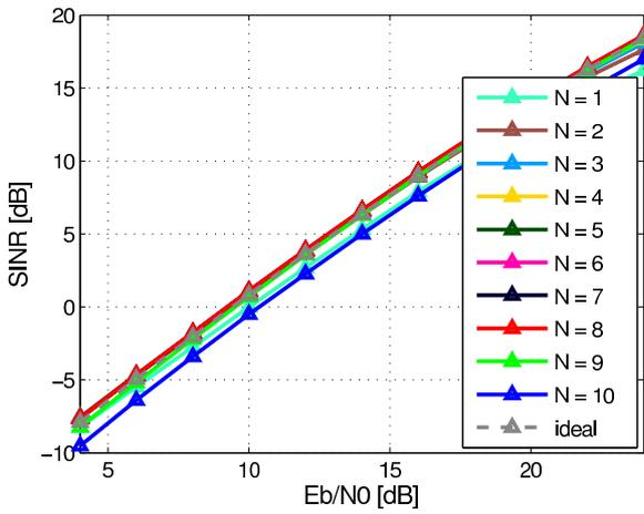
(a) SINR of MC-AcR with Bessel-Only filter approximation.
