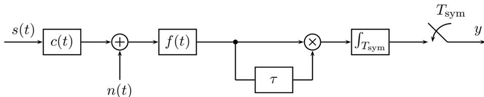
Figure 1.4: Signal flow diagram of an autocorrelation receiver.
