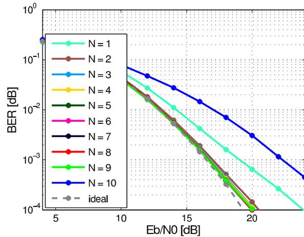
(f) BER of MC-MFED with Bessel-Only filter approximation.
