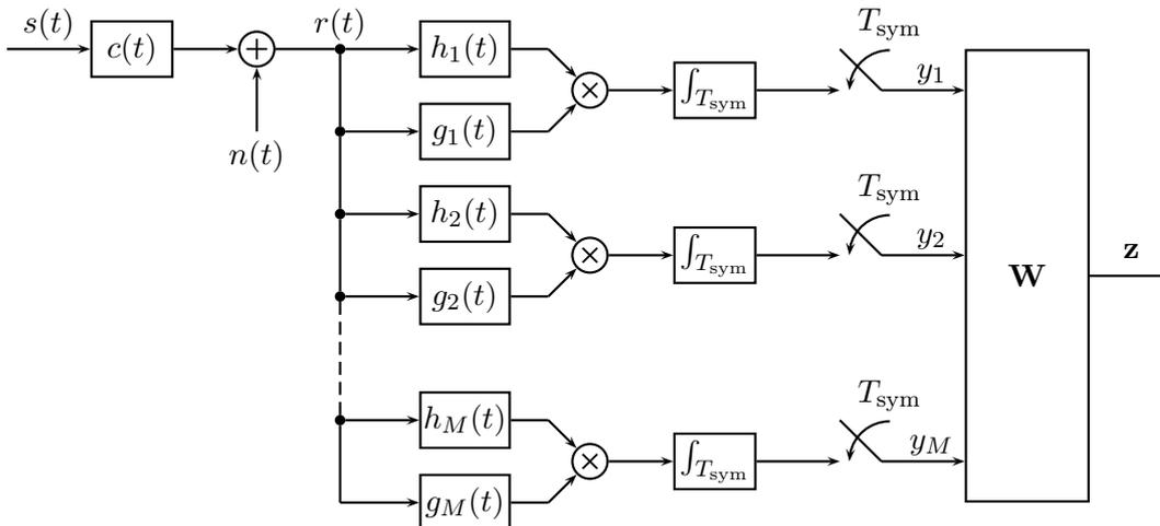
Figure 2.1: Signal flow diagram of a Generalized Noncoherent Multi-Channel Receiver.
