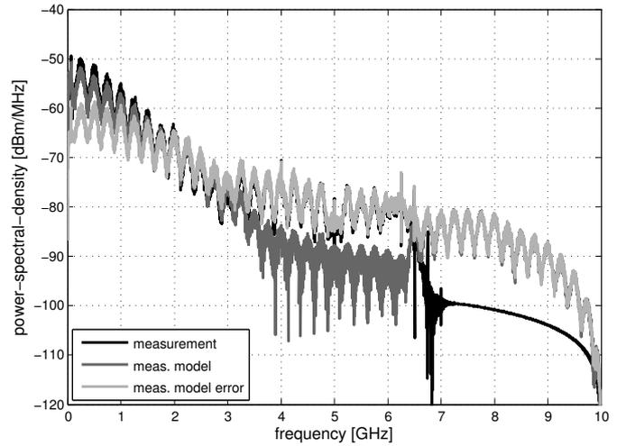
Fig. 9. Frequency domain output signals of the measurement-fitted system model in comparison to the measurement and the model error.
