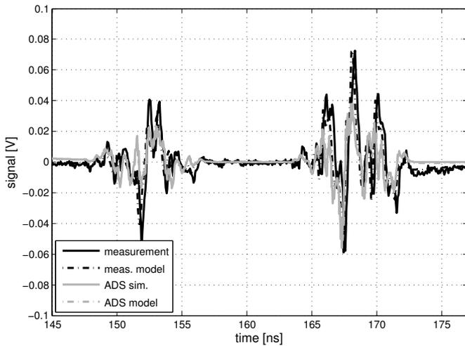
Fig. 8. Time domain output signals of the nonideal multiplier system model in comparison to the measurement, the output signal of the ADS circuit model, and the system model fitted onto the ADS circuit model.
