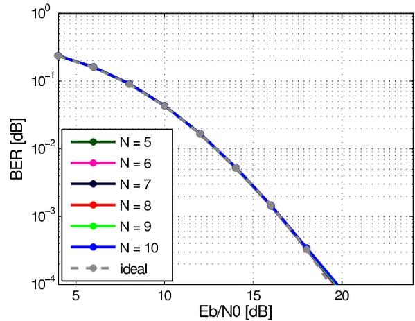
(f) BER of MC-MFED with Bessel-Notch filter approximation.
