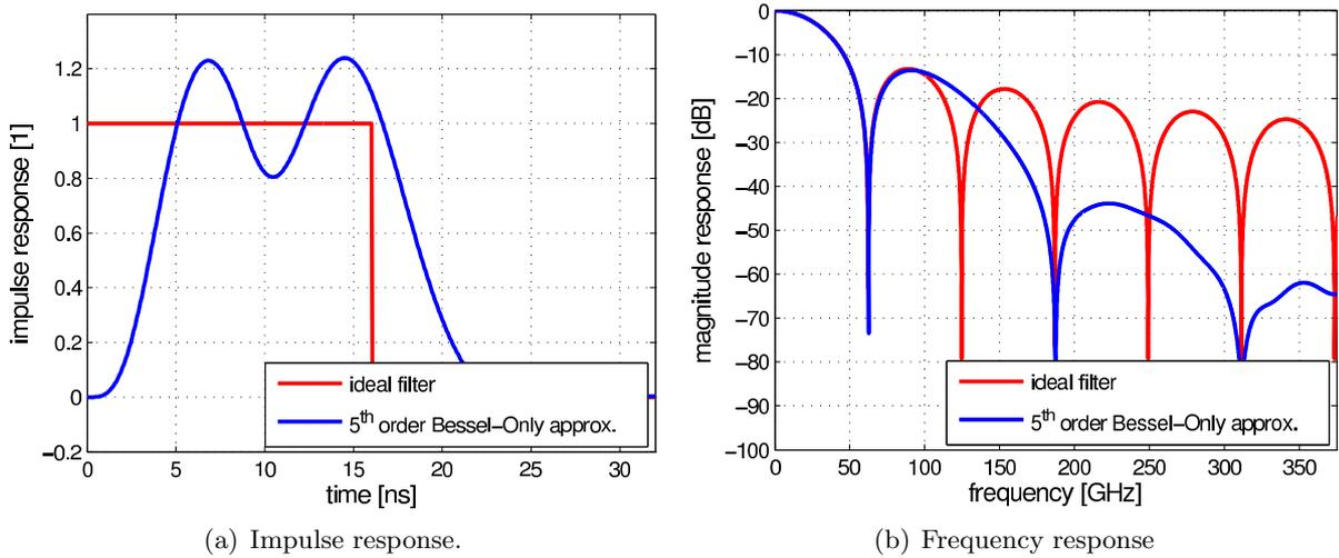
Figure 5.9: The mixed-signal impulse and magnitude response of the sliding window integration filter.
