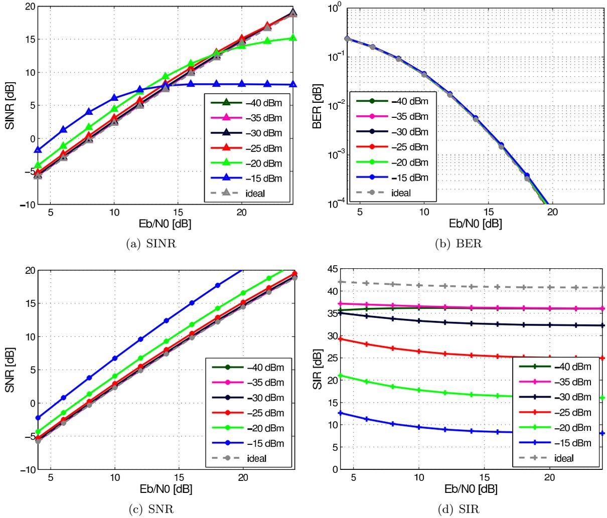
Figure D.7: SINR, SNR, SIR, and BER of the MC-MFED simulation-fitted multiplier model.
