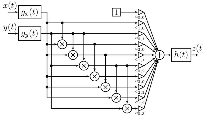
Figure 3.8: A nonideal multiplier system  $z(t) = \mathcal{M}\{x(t), y(t)\}$  of order  $U = 3$  consists of two input filters and one output filter, and seven ideal multipliers and gains, which model the static bivariate nonlinearity.
