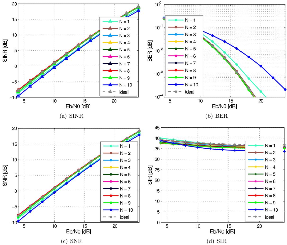
Figure D.11: SINR, SNR, SIR, and BER of the MC-ED with various filter orders  $N$  of Bessel-Only filter approximations.
