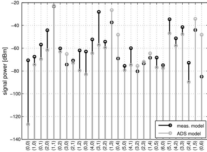
Fig. 11. Power of the nonlinear signal with the respective coefficients  $\{c_{u-v,v}\}$  of the system model fitted to the measurement and the system model fitted to the ADS simulation. The pair (a,b) represents its respective nonlinear coefficient  $c_{a,b}$ .
