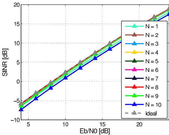
(e) SINR of MC-MFED with Bessel-Only filter approximation.
