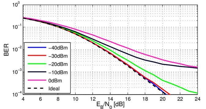
Fig. 8. Bit-error rate for various input power levels.
