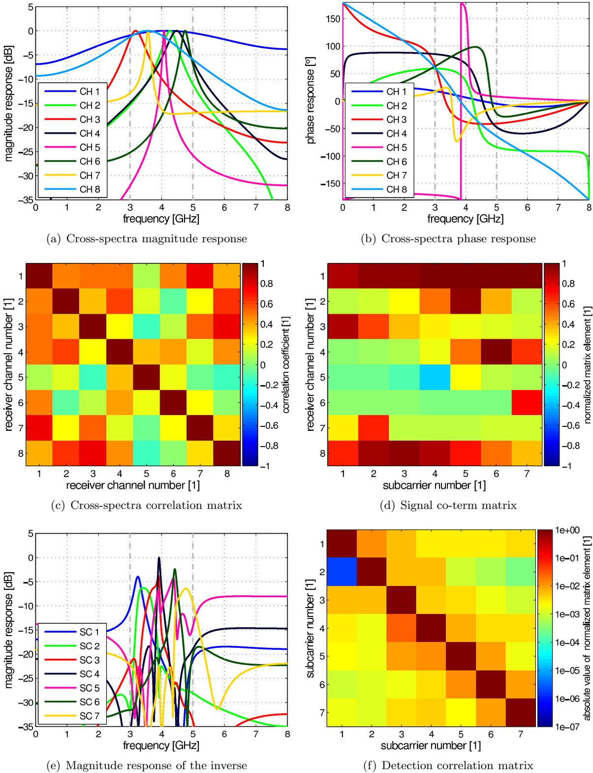
Figure D.2: Frequency response, Correlation matrix, and signal co-term matrix  $\mathbf{P}$  of an alternative (alt. 1) projection filter cross-spectra of 2<sup>nd</sup> order. The shown cross-spectra do have a condition number of  $\text{cond}\{\mathbf{P}\} = 16.78$ .
