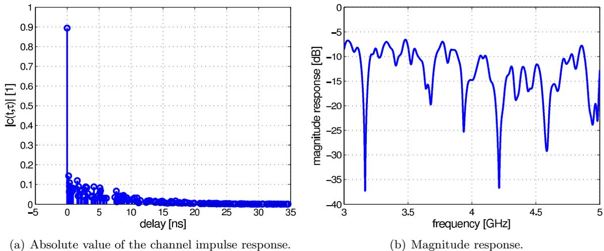
Figure A.1: Example of a time-variant multipath channel at given time  $t$ .
