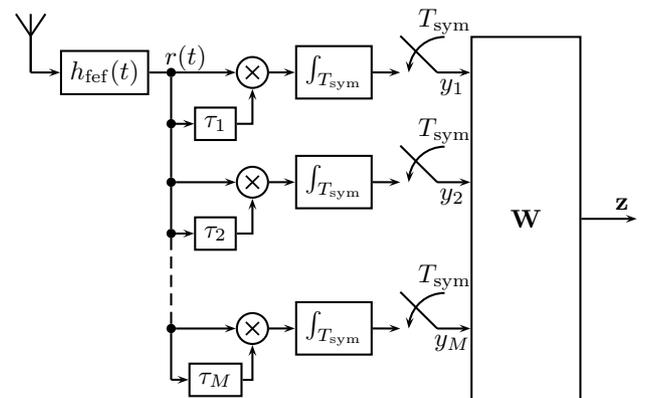
Fig. 1. The multichannel AcR architecture consists of delay filters, multiplication devices, and integration filters.
