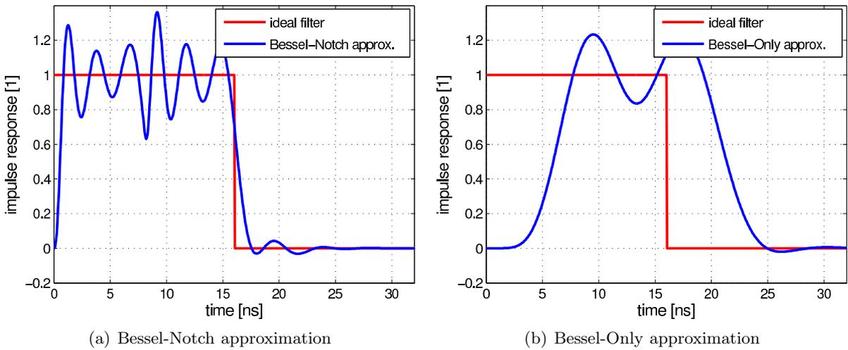
Figure 3.19: Impulse response of the Bessel-Notch approximation and Bessel-Only approximation sliding window integrator with 8<sup>th</sup> filter order.
