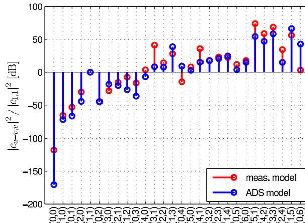
Figure 3.12: Polynomial coefficients  $\{c_{u-v}\}$  of the system models fitted to the measurement and to the ADS simulation, respectively. The coefficients are normalized to the desired signal coefficient  $c_{1,1}$ . The pair  $(a,b)$  represents the respective polynomial coefficient  $c_{a,b}$ .
