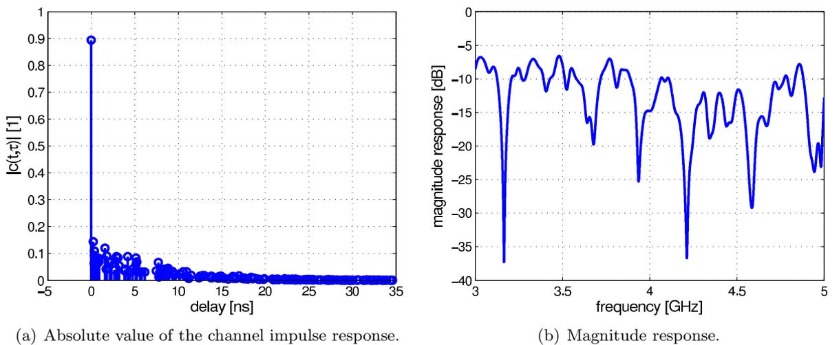
Figure 1.1: Example of a time-variant multipath channel at given time  $t$ .
