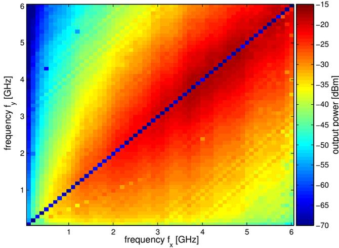
Fig. 5. Magnitude response of two dimensional frequency sweep measurements. Each grid point represents the output power of the output single-tone at a frequency of  $|f_x - f_y|$ , where  $f_x$  and  $f_y$  are frequencies of the input single-tones.
