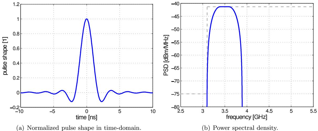
Figure 1.2: The IEEE 802.15.4a reference pulse. The pulse shape is a root raised-cosine pulse with a pulse width of  $T_p = 2$  ns and  $\beta = 0.6$ .
