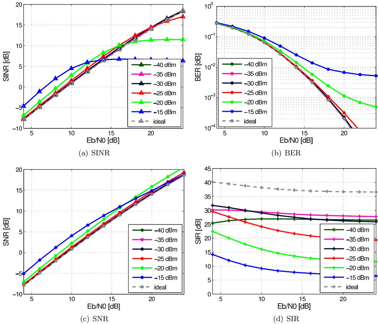
Figure D.5: SINR, SNR, SIR, and BER of the MC-AcR simulation-fitted multiplier model.
