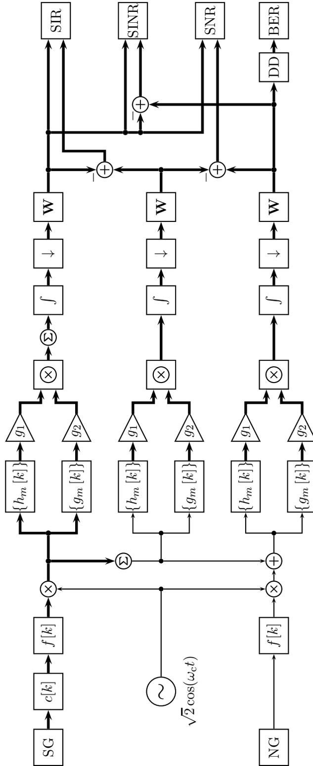
Figure 2.5: Signal flow diagram of the simulation framework.
