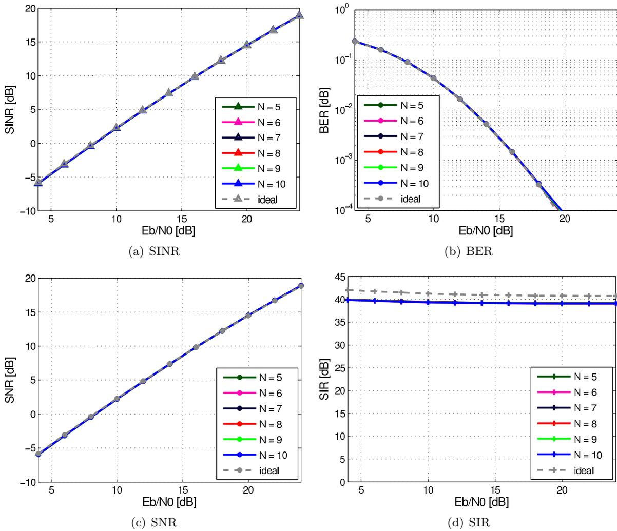
Figure D.12: SINR, SNR, SIR, and BER of the MC-ED with various filter orders  $N$  of Bessel-Notch filter approximations.
