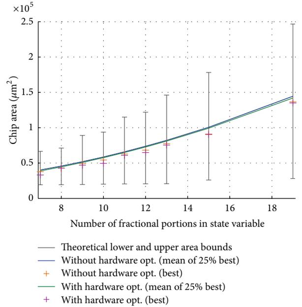
FIGURE 14: Chip area for predefined coefficients with and without multiobjective optimisation for hardware efficiency (fixed-point) as presented in Table 5. Limit bars indicate the theoretical minimum and maximum area requirements.
