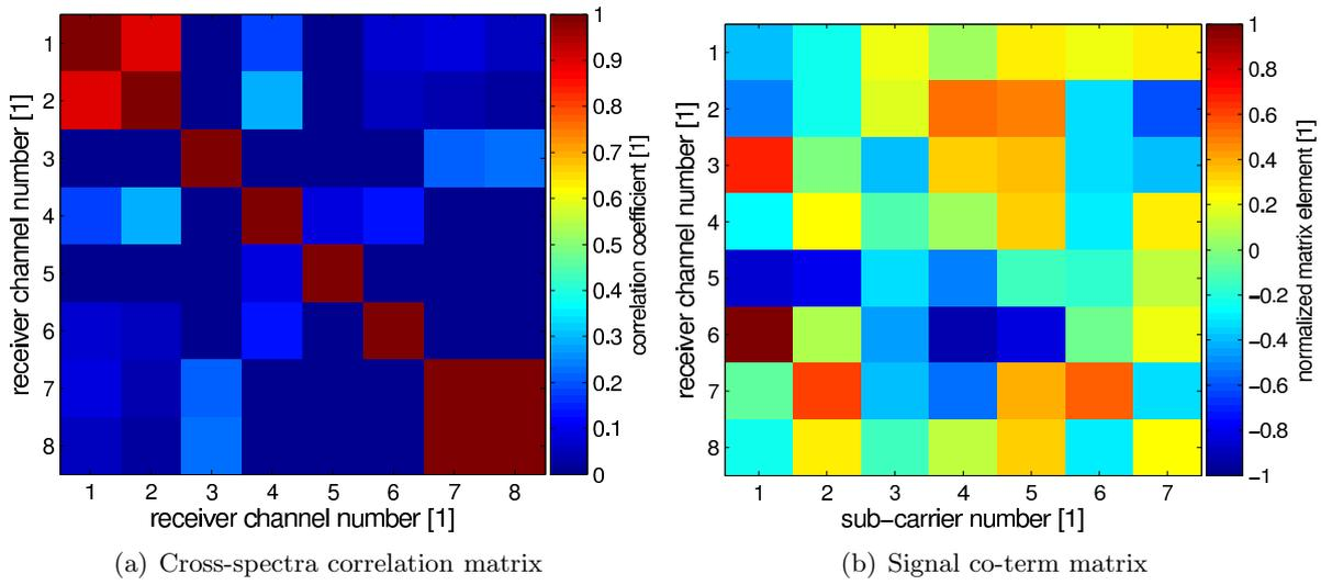
Figure 5.6: Correlation matrices of the LTCC filter cross-spectra and signal co-term matrix  $\mathbf{P}$  ( $\text{cond}\{\mathbf{P}\} = 13.86$ ) for  $M = 8$  channels.
