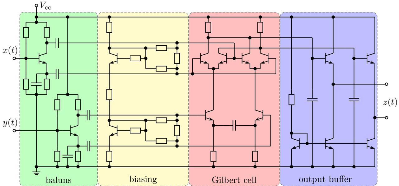
Figure 3.7: Circuit model of the UWB mixer designed by Ulm University consisting of two active single-ended-to-differential converter input stages (baluns), biasing, a four-quadrant Gilbert cell multiplier, and an output buffer.
