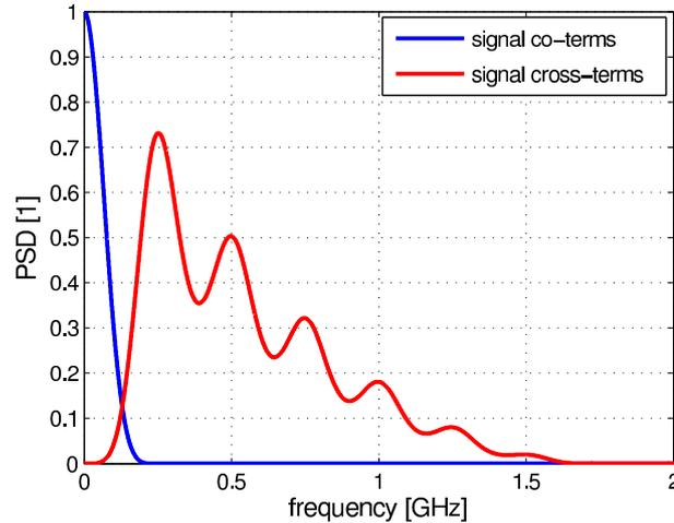
Figure 3.22: Power spectrum density of the signal co- and cross-terms of an NOFDM transmission scheme after the multiplication in a ProjR channel for  $K = 7$  subcarrier NOFDM signaling scheme.
