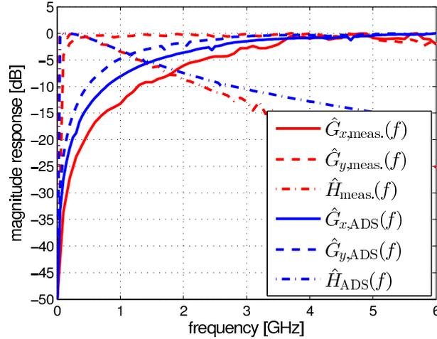
Figure 3.11: Input and output filter magnitude responses of the system model fitted to the measurement and to the ADS circuit model simulation.
