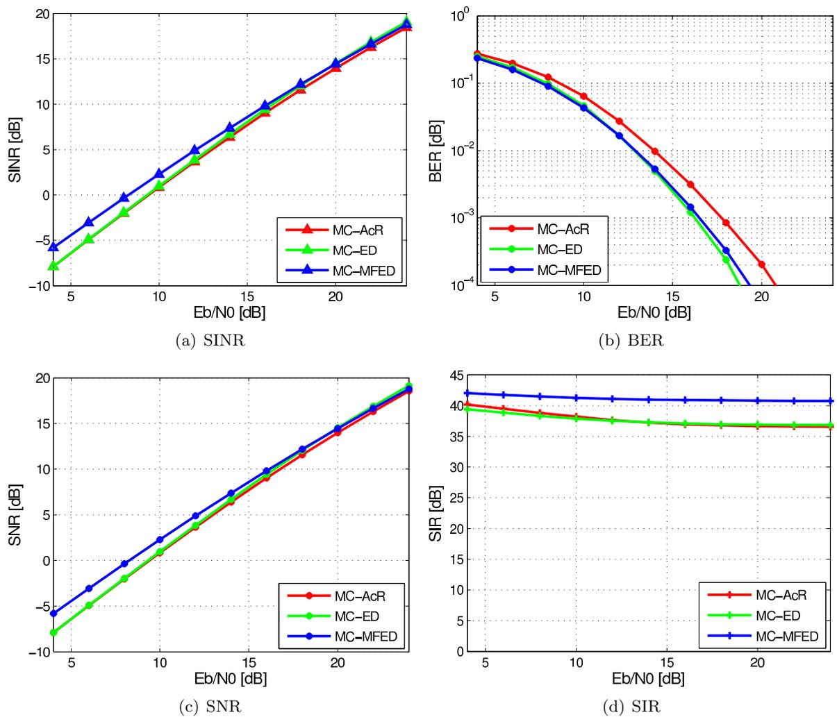
Figure 2.12: SINR, SNR, SIR, and BER of the MC-AcR, the MC-ED, and the MC-MFED.
