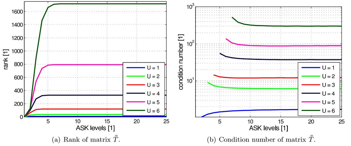
Figure 4.1: Rank and condition number of matrix  $\bar{T}$  for various ASK levels and order  $U$  of nonlinearity.
