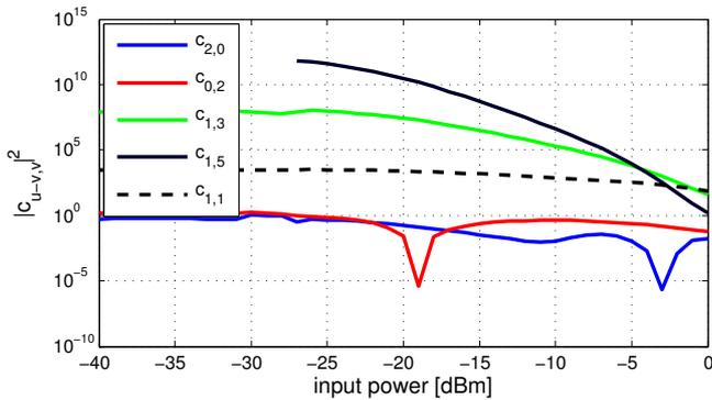
Fig. 3. Coefficients of the static nonlinearity.
