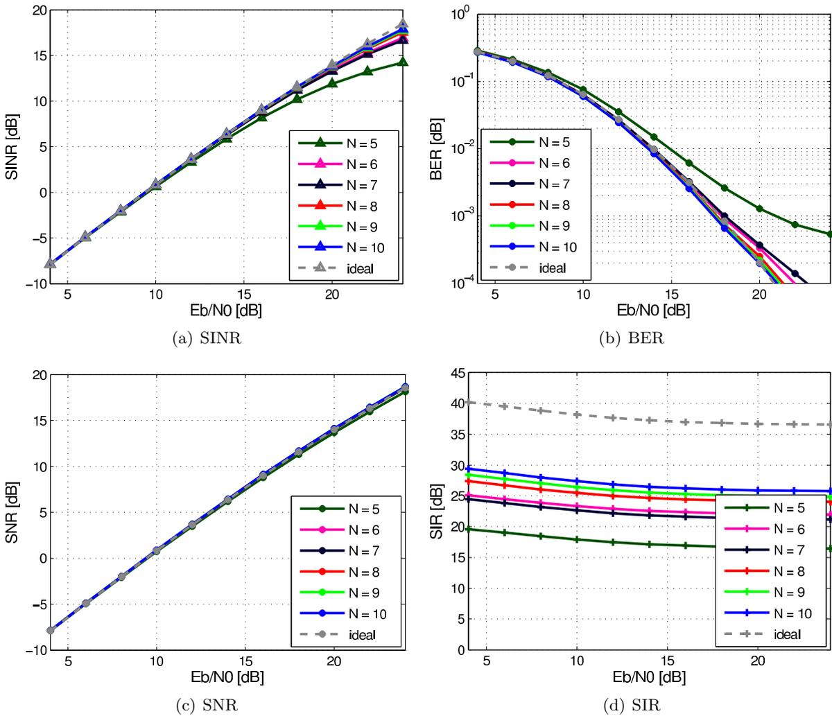
Figure D.8: SINR, SNR, SIR, and BER of the MC-AcR with various filter orders  $N$  of Bessel-Notch filter approximations.
