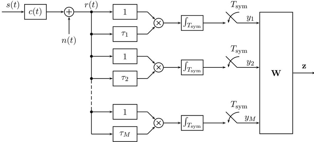
Figure 2.10: Signal flow diagram of the Multi-Channel Autocorrelation Receiver.
