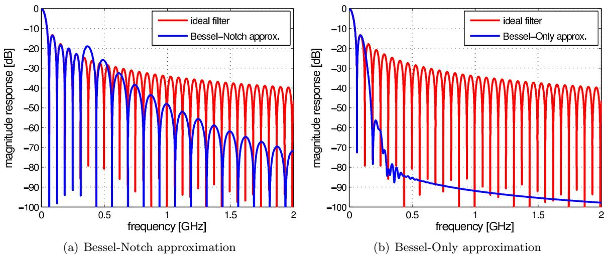
Figure 3.20: Magnitude response of the Bessel-Notch approximation and Bessel-Only approximation sliding window integrator with 8<sup>th</sup> filter order.
