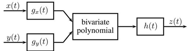
Fig. 1. Wiener-Hammerstein system model consisting of input filters  $g_x(t)$  and  $g_y(t)$ , an output filter  $h(t)$ , and a bivariate polynomial as static nonlinearity.
