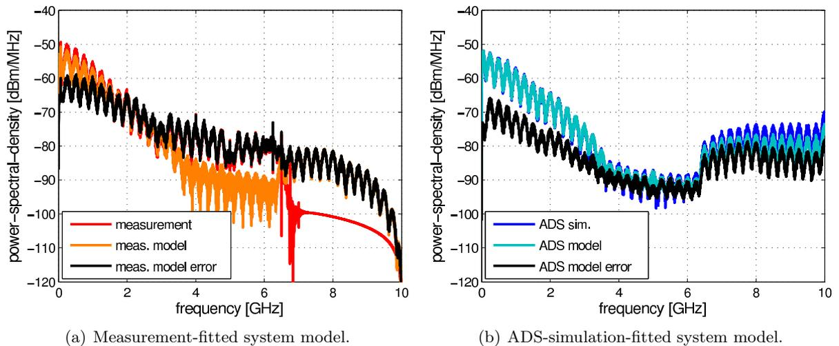
Figure 3.14: Frequency domain output signals in comparison to the ADS circuit model and the model error.
