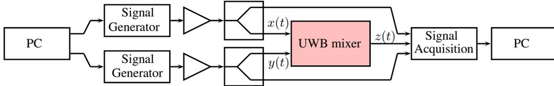
Figure 3.9: Measurement setup for mixer identification.
