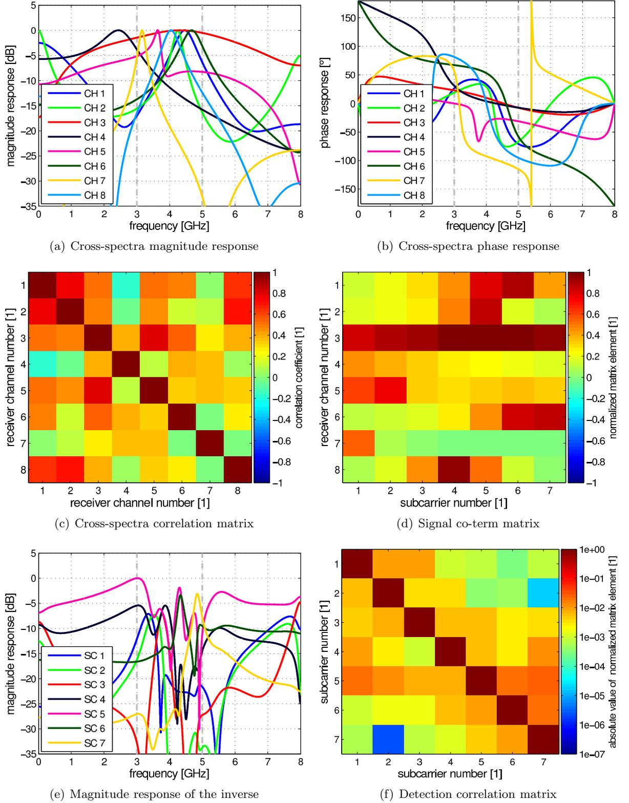
Figure 3.3: Frequency response, Correlation matrix, and signal co-term matrix  $\mathbf{P}$  of a projection filter cross-spectra of 4<sup>th</sup> order. The shown cross-spectra do have a condition number of  $\text{cond}\{\mathbf{P}\} = 25.53$ .
