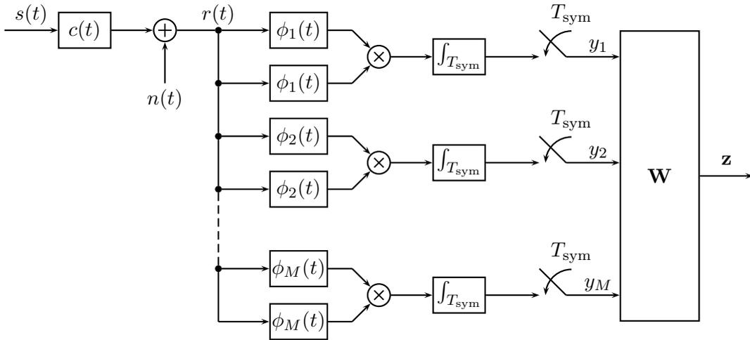
Figure 2.8: Signal flow diagram of the Multi-Channel Matched Filter Receiver.
