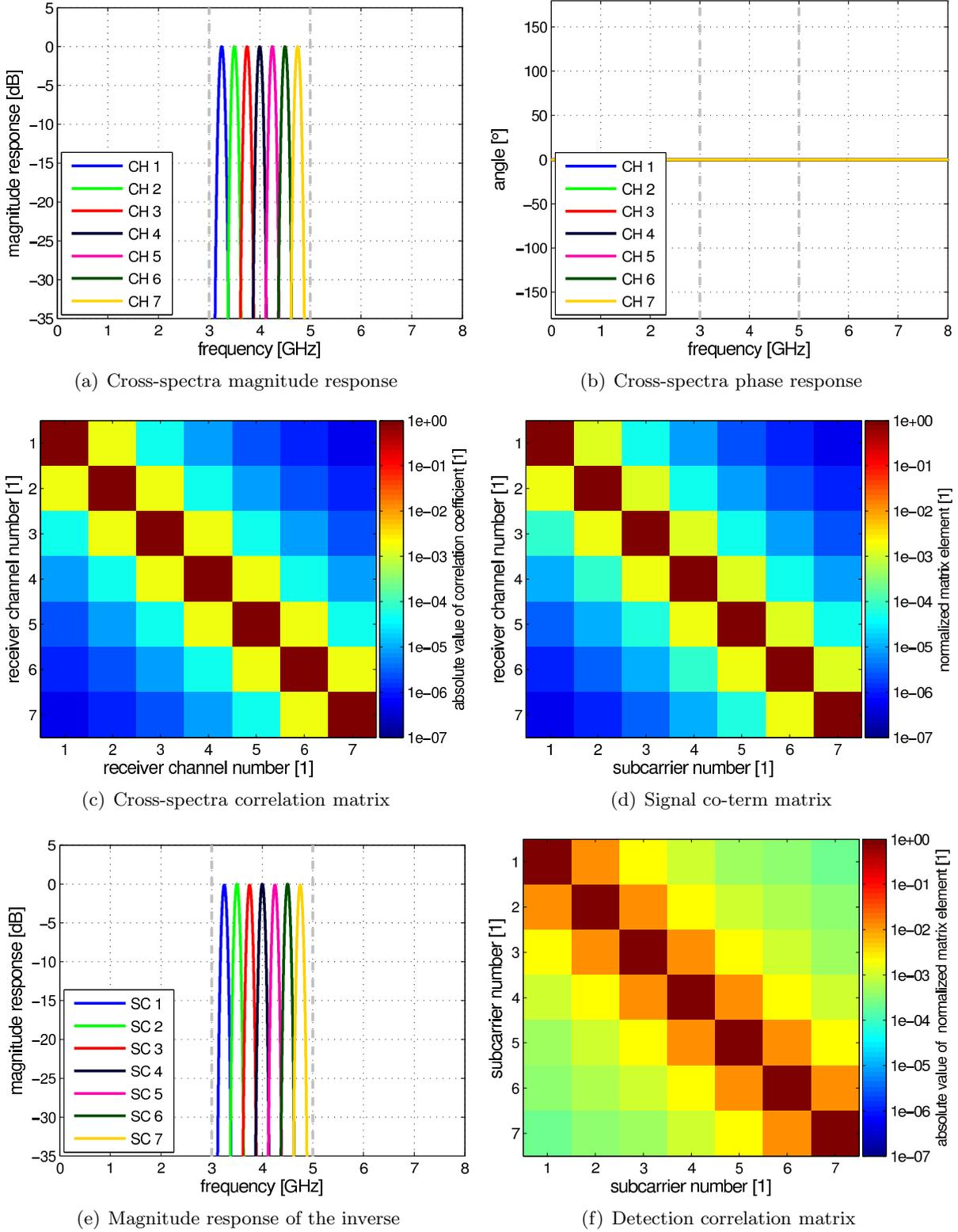
Figure 2.9: Projection filter cross-spectra, correlation matrices, signal co-term matrix  $\mathbf{P}$  ( $\text{cond}\{\mathbf{P}\} = 1.0175$ ), and spectra of the inverse of the MC-MFED for  $M = 7$  channels.
