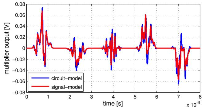
Fig. 4. Time domain output signals of the nonideal multiplier model in comparison to the output signal of the circuit model of five NOFDM pulses. The input signals had a power of  $-20$  dBm.
