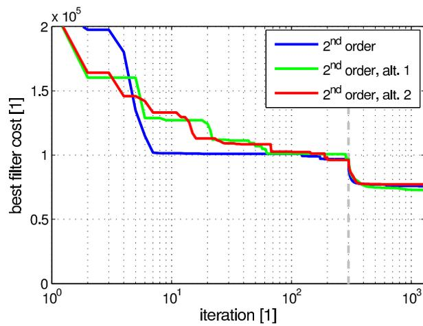
Figure D.1: Cost of best found filter per iteration of three 2<sup>nd</sup> order projection filter cross-spectra for a  $M = 8$  channel receiver.
