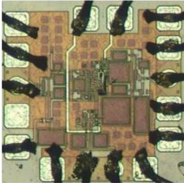
Figure 5.8: Micrograph of the UWB mixer die designed by Ulm University. (Picture taken from [99].)
