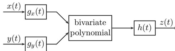
Figure 3.6: Wiener-Hammerstein system model consisting of input filters  $g_x(t)$  and  $g_y(t)$ , an output filter  $h(t)$ , and a bivariate polynomial as static nonlinearity.
