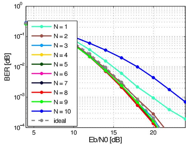
(b) BER of MC-AcR with Bessel-Only filter approximation.
