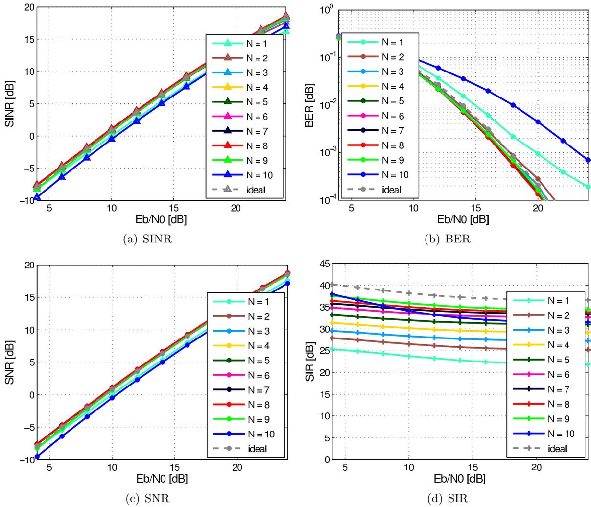
Figure D.9: SINR, SNR, SIR, and BER of the MC-AcR with various filter orders  $N$  of Bessel-Only filter approximations.
