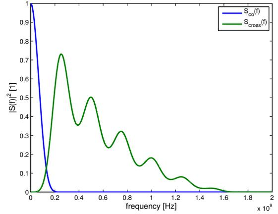
Fig. 2. Power spectrum density of the co- and cross-terms of an OFDM transmission scheme after the multiplication in an AcR channel for  $K = 7$  sub-carrier UWB OFDM signaling scheme.
