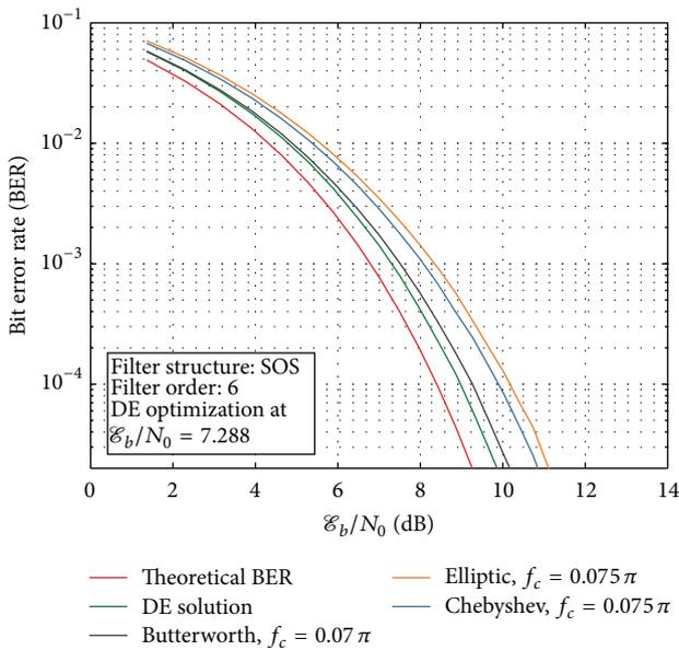
FIGURE 9: Transceiver BER for the optimum solution found by the DE algorithm at an operation point of  $\mathcal{E}_b/N_0 = 7.288$ . Butterworth, elliptic, and Chebyshev filters are plotted as reference.  $N_b = 10^6$  bits.
