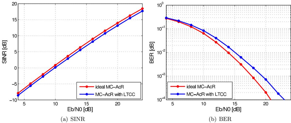
Figure 5.7: SINR and BER of the MC-AcR with LTCC filters.
