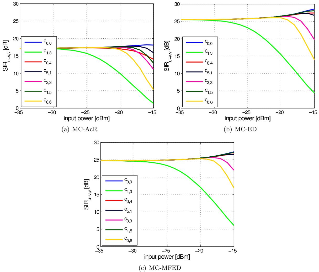
Figure 3.16:  $SIR_{u-v,v}$  for various nonlinear terms of different noncoherent multi-channel receivers.
