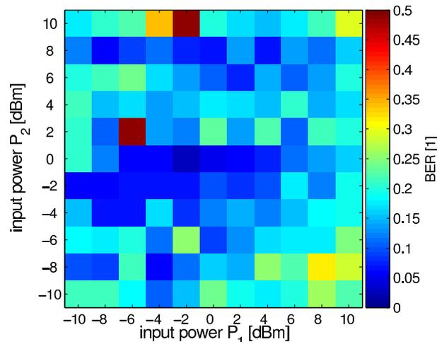
Figure 5.10: Measured BER for various LTCC input powers.
