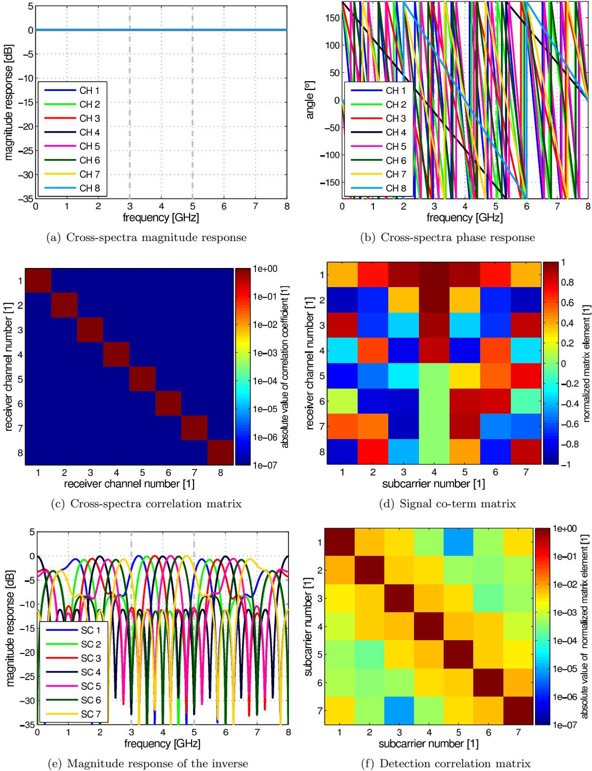
Figure 2.11: Projection filter cross-spectra, correlation matrices, signal co-term matrix  $\mathbf{P}$  ( $\text{cond}\{\mathbf{P}\} = 1.1519$ ), and spectra of the inverse of the MC-AcR for  $M = 8$  channels.
