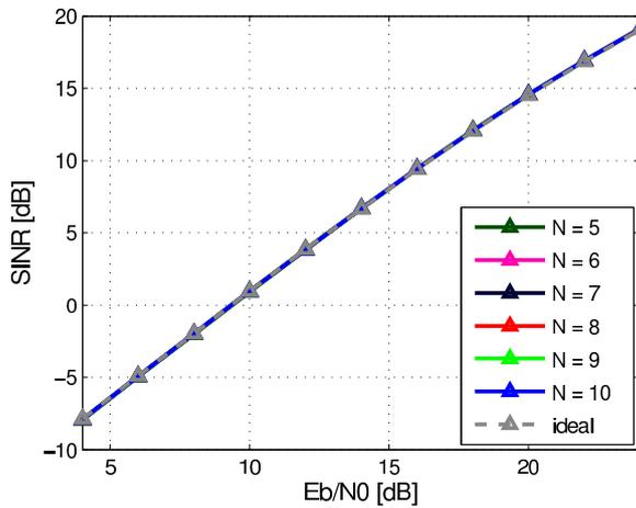
(c) SINR of MC-ED with Bessel-Notch filter approximation.
