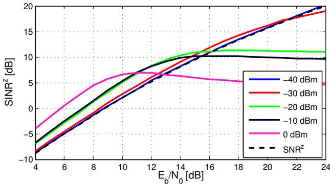
Fig. 7. Signal-to-interference-and-noise ratio for various input power levels.
