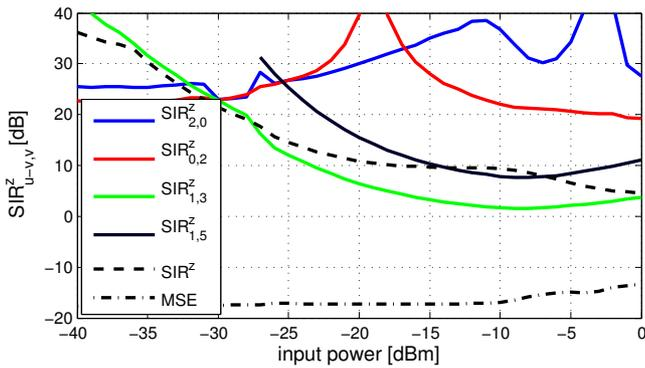
Fig. 6. Signal-to-interference ratio for various nonlinear terms.
