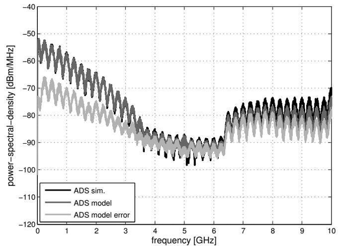
Fig. 10. Frequency domain output signals of the ADS-simulation-fitted system model in comparison to the ADS circuit model and the model error.
