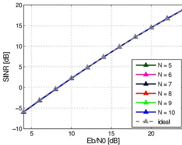
(e) SINR of MC-MFED with Bessel-Notch filter approximation.
