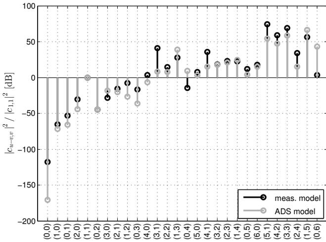
Fig. 7. Polynomial coefficients  $\{c_{u-v,v}\}$  of the system models fitted to the measurement and to the ADS simulation, respectively. The coefficients are normalized to the desired signal coefficient  $c_{1,1}$ . The pair  $(a, b)$  represents the respective polynomial coefficient  $c_{a,b}$ .
