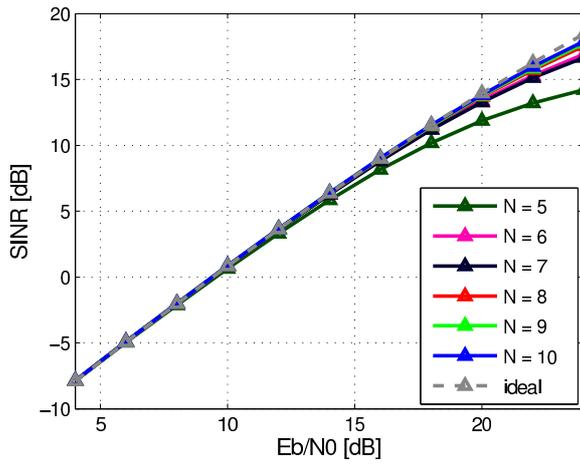
(a) SINR of MC-AcR with Bessel-Notch filter approximation.
