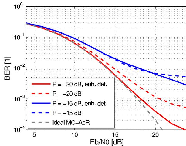
Figure 4.3: BER of the non-enhanced and enhanced detection with mixer input power of  $-20$  dBm ( $U = 2$ , 3 ASK levels, 4000 symbols) and  $-15$  dB ( $U = 6$ , 7 ASK levels, 12000 symbols).
