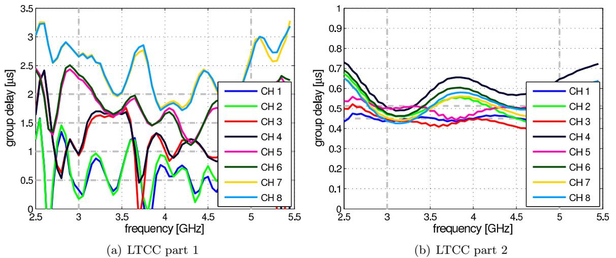
Figure 5.5: Group delay of the LTCC filters.
