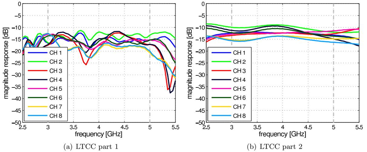
Figure 5.4: Magnitude response of the LTCC delay line filters.
