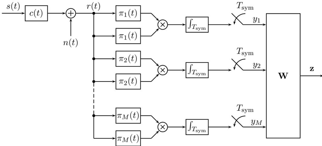
Figure 2.6: Signal flow diagram of the Multi-Channel Energy Detector.
