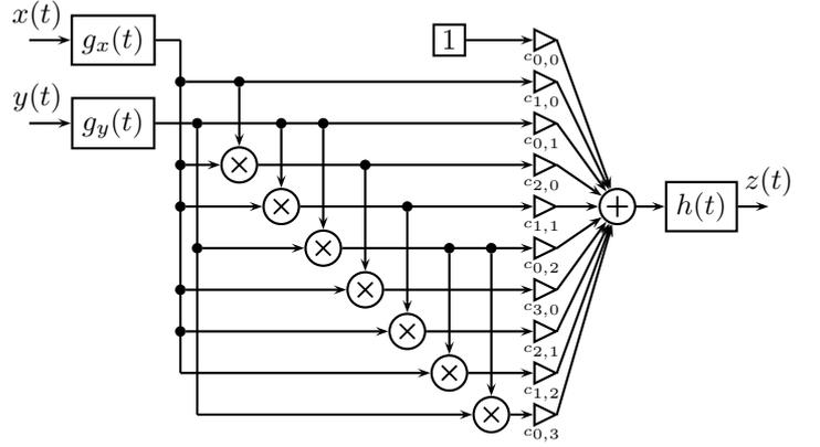
Fig. 3. A nonideal multiplier system  $z(t) = \mathcal{M}\{x(t), y(t)\}$  of order  $U = 3$  consists of two input and one output filters, and seven ideal multipliers and gains, which model the static bivariate nonlinearity.
