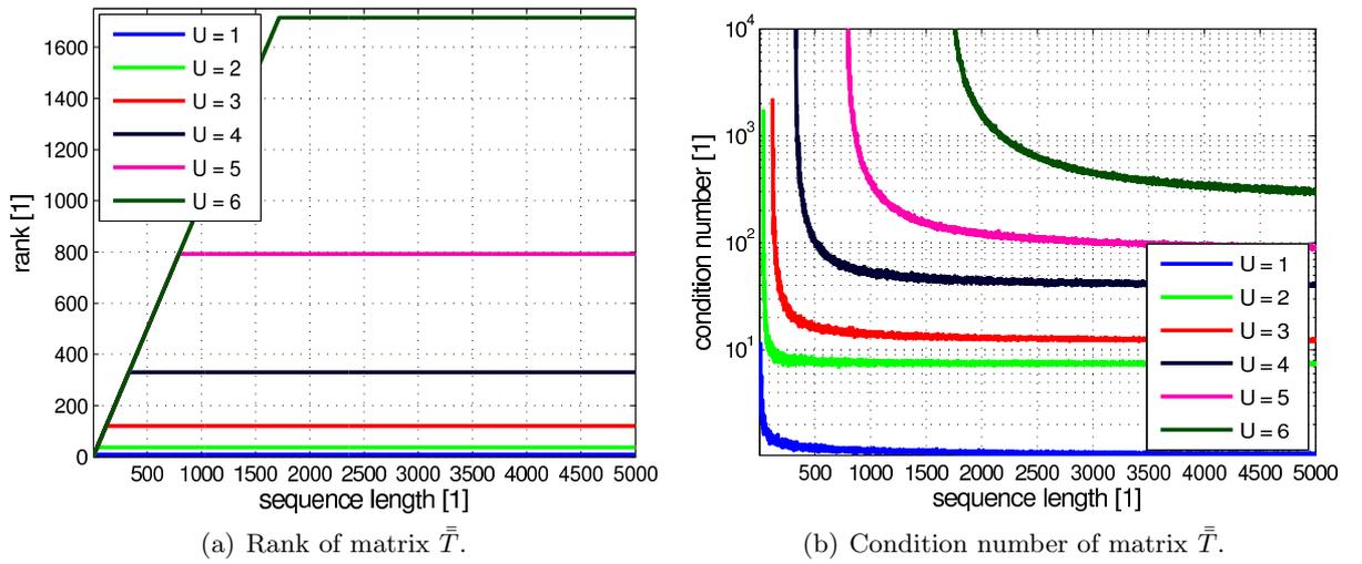
Figure 4.2: Rank and condition number of matrix  $\bar{T}$  for various sequence lengths and order  $U$  of nonlinearity.
