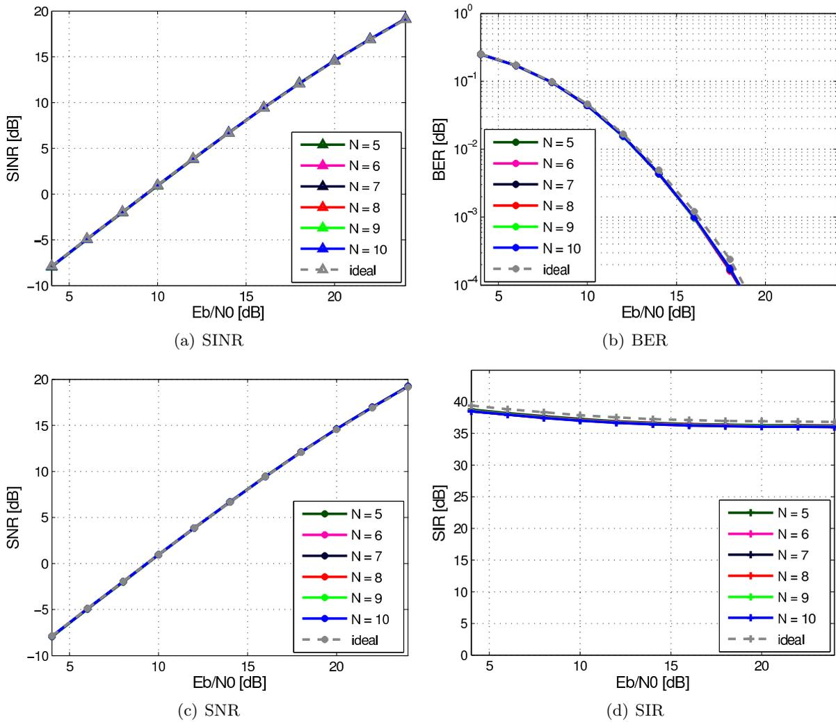
Figure D.10: SINR, SNR, SIR, and BER of the MC-ED with various filter orders  $N$  of Bessel-Notch filter approximations.
