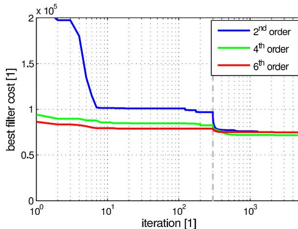
Figure 3.1: Cost of best found filter per iteration of different order of projection filter cross-spectra for a  $M = 8$  channel receiver.
