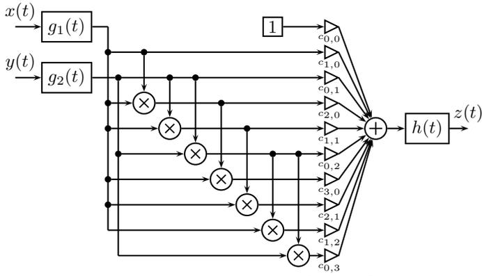
Fig. 2. A nonideal multiplier system  $z(t) = \mathcal{M}\{x(t), y(t)\}$  of order  $U = 3$  consists of two input and one output filters, and seven ideal multipliers and gains, which model the static bivariate nonlinearity.
