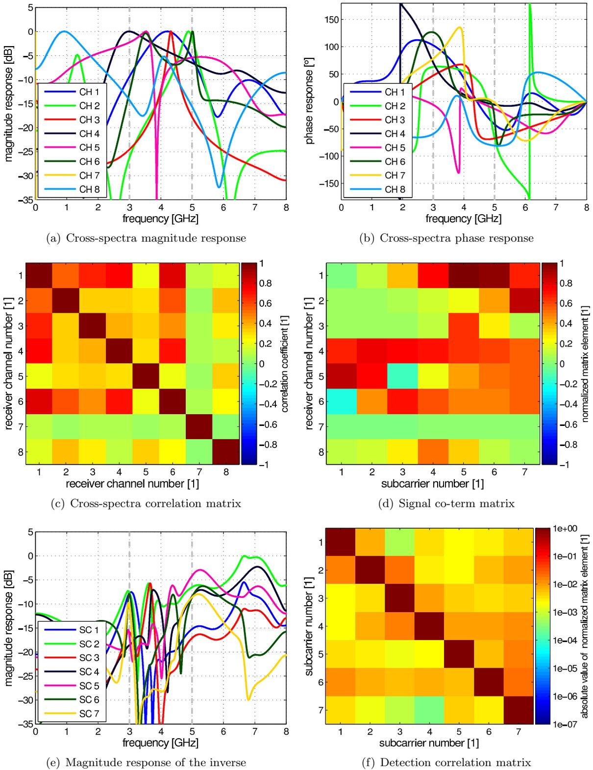
Figure 3.4: Frequency response, Correlation matrix, and signal co-term matrix  $\mathbf{P}$  of a projection filter cross-spectra of 6<sup>th</sup> order. The shown cross-spectra do have a condition number of  $\text{cond}\{\mathbf{P}\} = 19.35$ .
