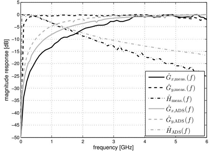
Fig. 6. Input and output filter magnitude responses of the system model fitted to the measurement and to the ADS circuit model simulation.
