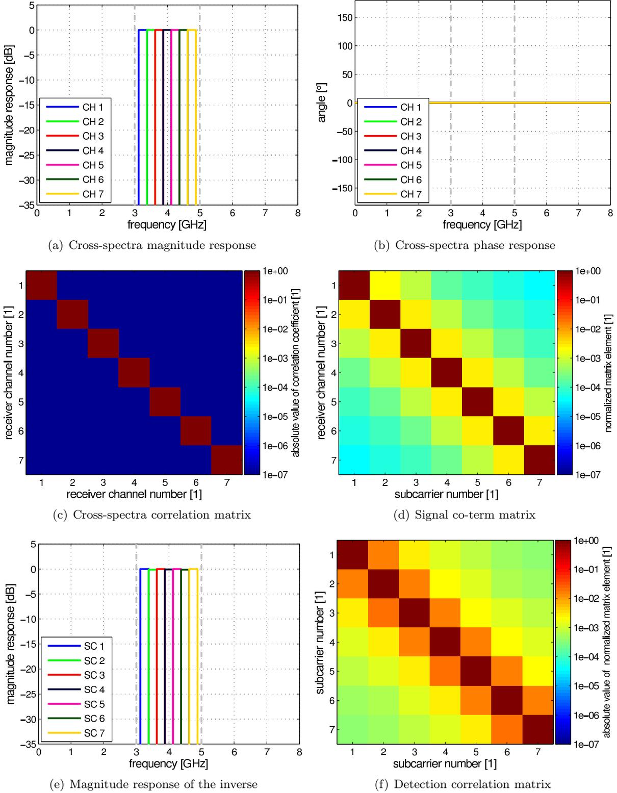
Figure 2.7: Projection filter cross-spectra, correlation matrix, signal co-term matrix  $\mathbf{P}$  ( $\text{cond}\{\mathbf{P}\} = 1.0187$ ), and spectra of the inverse of the MC-ED projection for  $M = 7$  channels.
