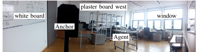
Fig. 2. Picture of the measured room. The anchor and agent positions as well as the surfaces generating the analyzed MPCs are labeled (cf. Fig. 1).
