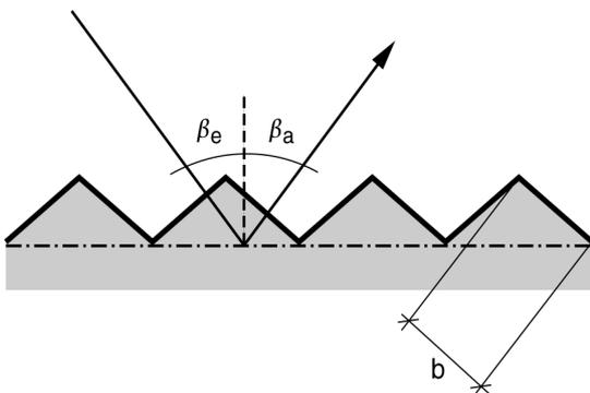
$\lambda > b$  : In this case, the wall behind the sub surfaces reflects the wave according to the geometrical reflection lemma  $\beta_e = \beta_a$
