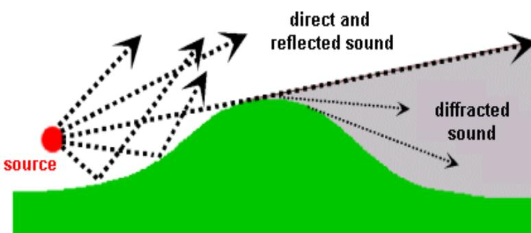
*Picture 1.7 :Diffraction on an obstacle*
