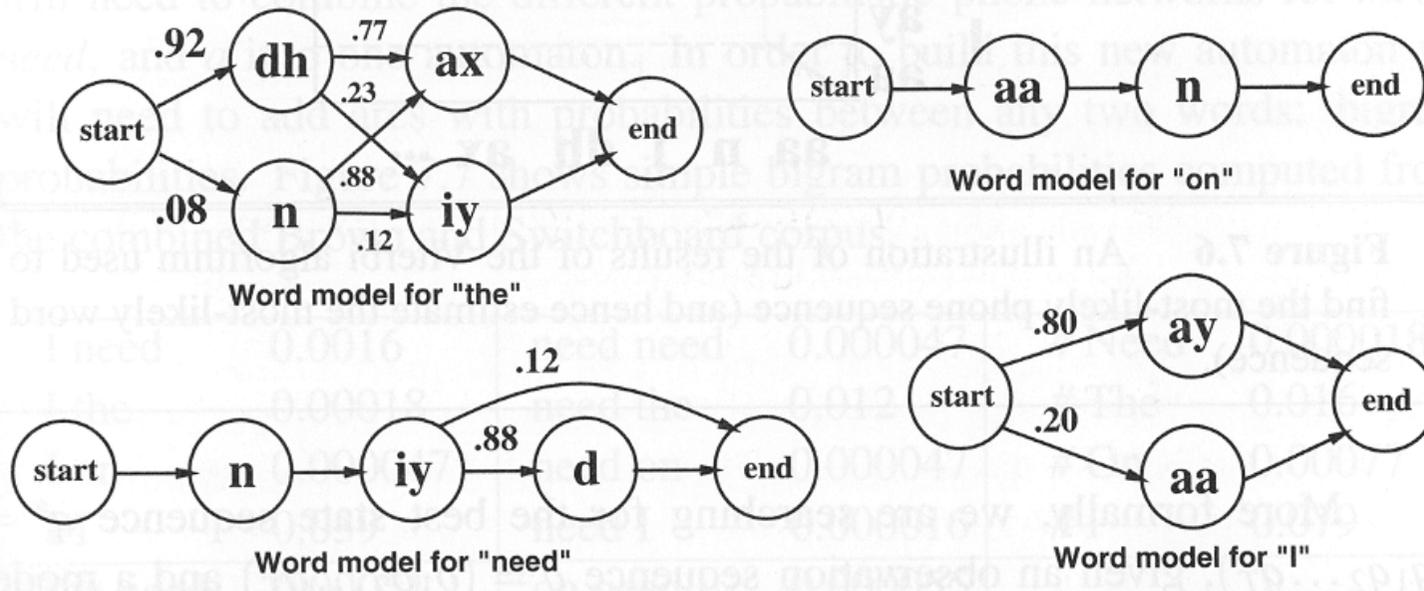
Viterbi algorithm used to find the most-likely phone sequence within word models:
