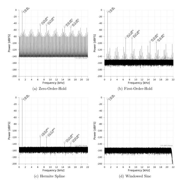
Figure 4.8: Harmonic Distortion test result.
