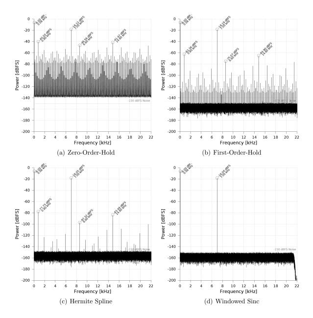
Figure 4.9: Intermodulation Distortion test result.
