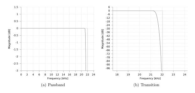
Figure 4.4: Magnitude of the frequency response of the windowed sinc.
