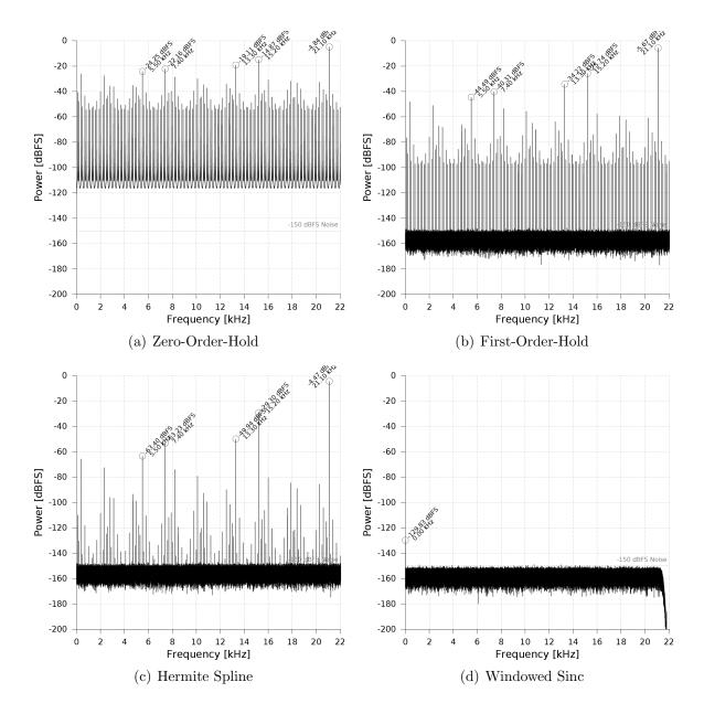
Figure 4.7: Aliasing test result.
