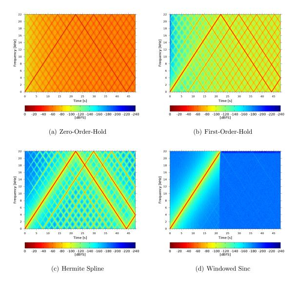
Figure 4.6: Sweep test result.
