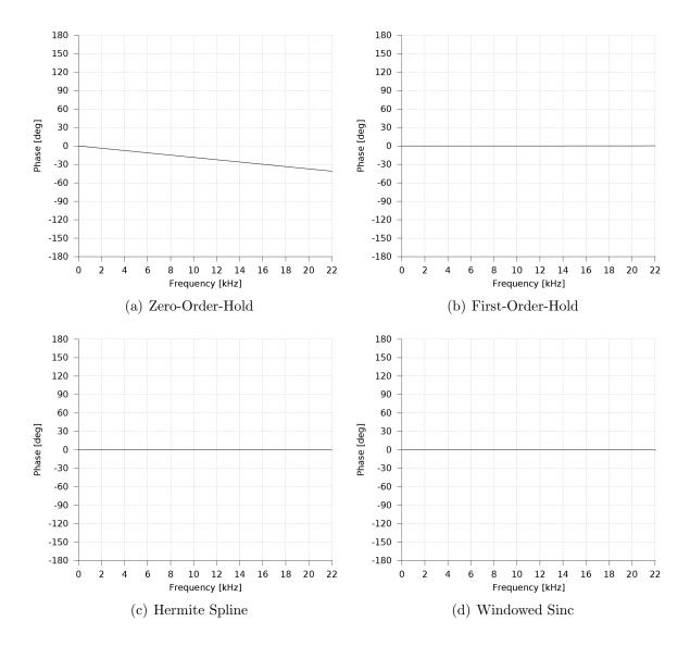
Figure 4.2: Phase of the frequency response.
