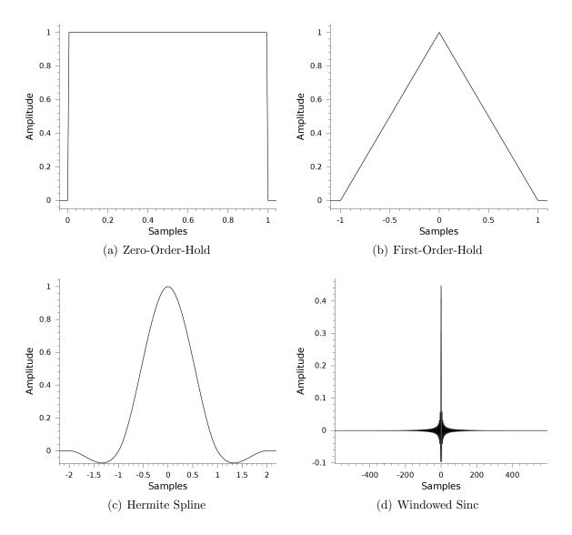
Figure 4.1: Impulse response in the time domain.
