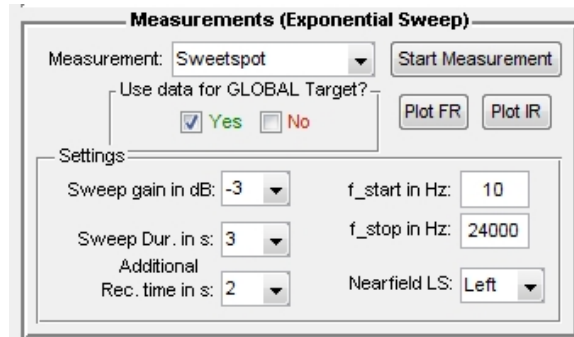
Figure 20.3.: RoLoSpEQ: Measurement (Exponential Sweep). In the drop-down list several measurement positions can be selected. Additionally certain measurements can be activated for global RMS averaging (“Use data for global target?”). The measurement can be started with the button Start measurement . After each measurement the measured data set (left and right loudspeaker) is automatically activated for global RMS averaging and the measurement selector is automatically increased to the next measurement position.
