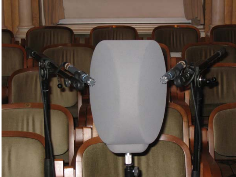
Figure 6.19: The binaural recording system "Source" [Graf, 1999] with 2 AKG micro-phones.
