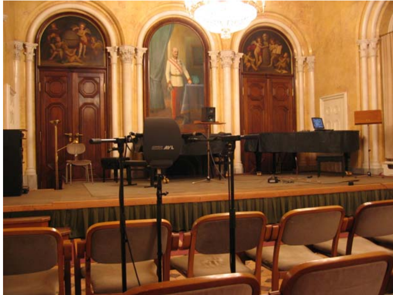
Figure 6.20: The loudspeaker is located on the stage and the binaural recording system is located on position 1.
