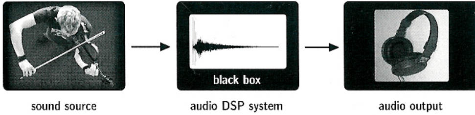
Figure 4.1: A source signal can be convolved with the room impulse response. The output can be listened to [Vorländer, 2008].
